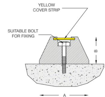
They are designed not to cause any damage to vehicles. KerbStopper Buffers give the drivers a clear warning that their rear wheels are parked correctly. They are supplied with Pre-drilled holes for concrete or asphalt installations.
